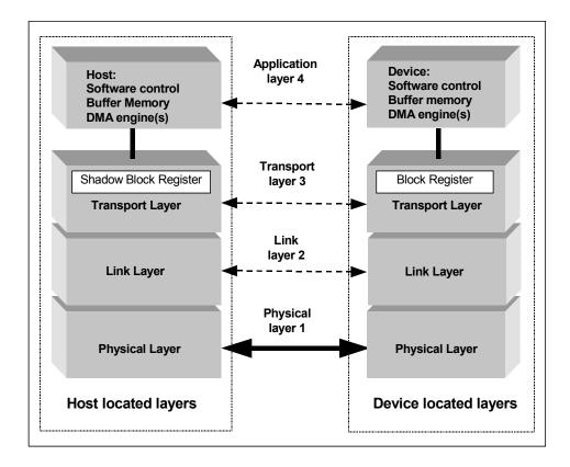
Figure 5.3 Conceptual diagram of communication layers
